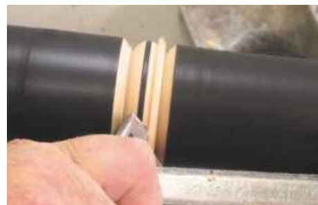
▲ Pic.18 I like to turn the main shape in one pass; this will generally give you the best opportunity for a good shape. Moving your body round as the tool advances will help to avoid catches
